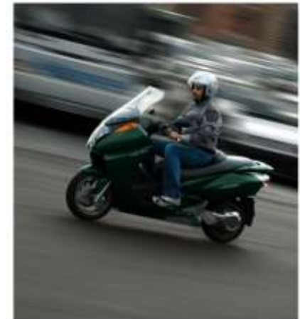
Figure 20.44. Vectrix: 2.75 kWh per 100 km. Photo from www.vectrix.com .
